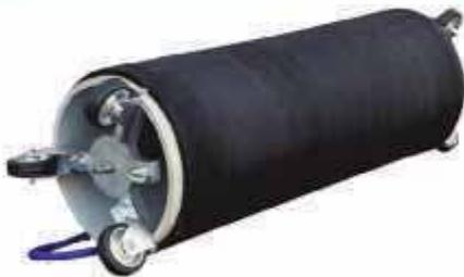
These are suitable for repair of pipeline joints or repair of shorter pipeline sections along with insertion of stainless steel shells. On each side of the packer three wheels are attached at an angle of 120 degrees to prevent tipping over while transported along the pipeline.
