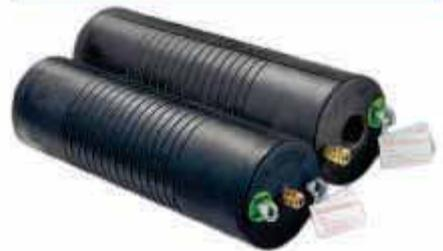
These all-purpose plugs have a superior surface pattern for sealing and are used for sealing and testing pipeline tightness with air or water. Multi-size plugs are stretchable so only a few plugs are required to cover pipelines of different diameters.
