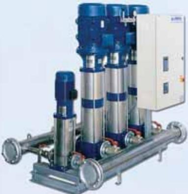
Variable speed water booster sets with wide range of 2, 3 and 4 multistage vertical electric pumps. Pump controlled by pressure switches with constant or variable speed operation. The range has been designed to supply water to users on an intermittent or variable basis using electric motors controlled by an electric panel.
