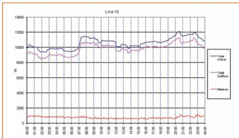
Figure 6 – Trunk main balance Line 10 showing effect of subtracting two large flows. Inconclusive result
