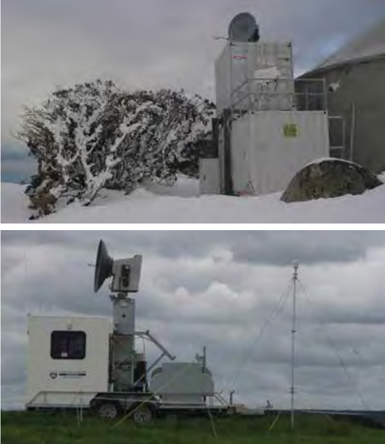
Figure 3 – University of Auckland radars. (Top) Constructed in a shipping container and sited overlooking a hydro power catchment in the Snowy Mountains of Australia (photo courtesy Andrew Peace). (Above) A towable trailer mounted radar overlooking the Waipapa catchment near the Waikato River.
