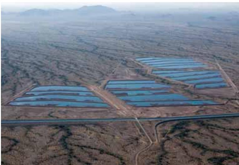
Figure 3 – Tonopah Desert recharge project (TDRP) comprising of nearly 90 ha of spreading basins (CAP 2011)
