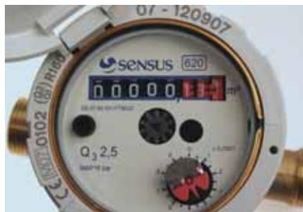
Meter register with OIML R49 R160 certification markings
