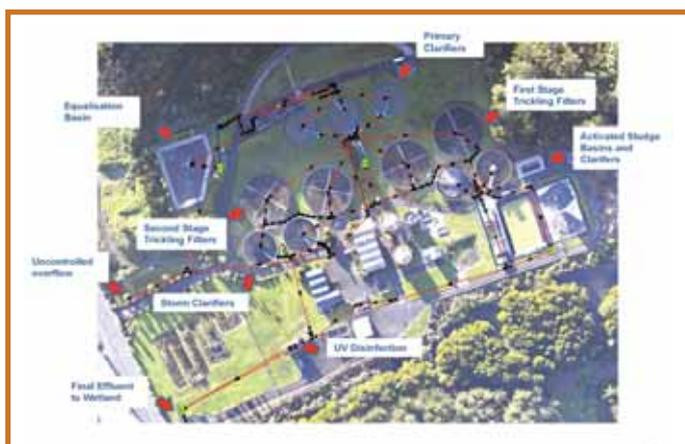
Figure 2 – Aerial of WWTP and key process units
