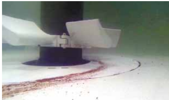
This underwater image demonstrates the forced hydraulic action of the PISTA® Vio™ and how it sweeps grit along the flat floor and enables capture of 95 percent of particles down to 105 microns (140 mesh).
