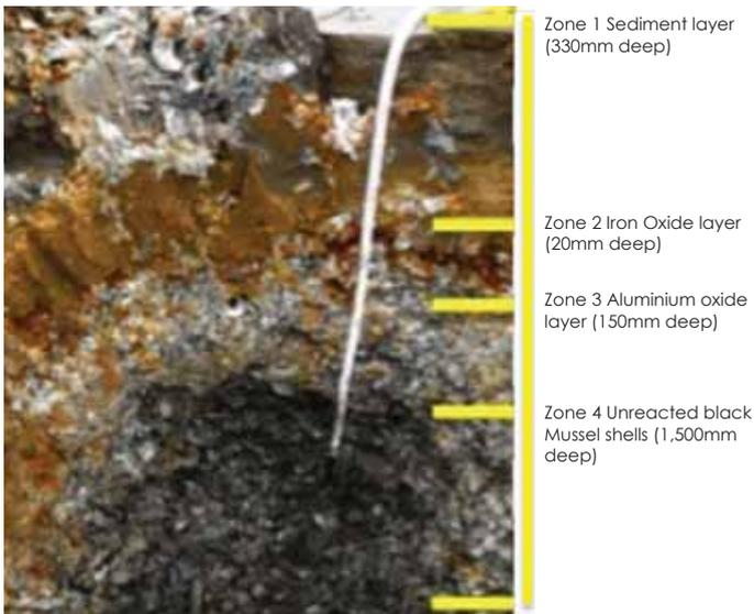
Photograph 2 – Cross section through the Manchester Street seep mussel shell bioreactor at Stockton coal mine on day 933. Four distinct zones are shown (sediment layer, iron oxide layer, mussel shell with aluminium oxide layer, and unreacted mussel shell) and the depth of each layer.
