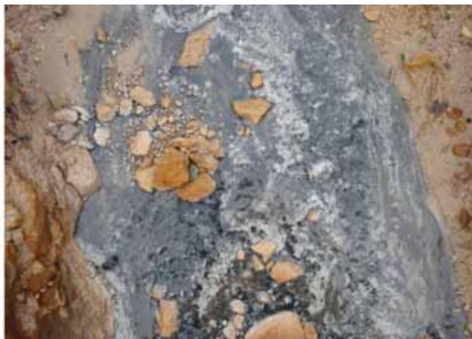
Photograph 1 – Black precipitate at the effluent discharge point for the Manchester Street seep mussel shell bioreactor at Stockton coal mine
