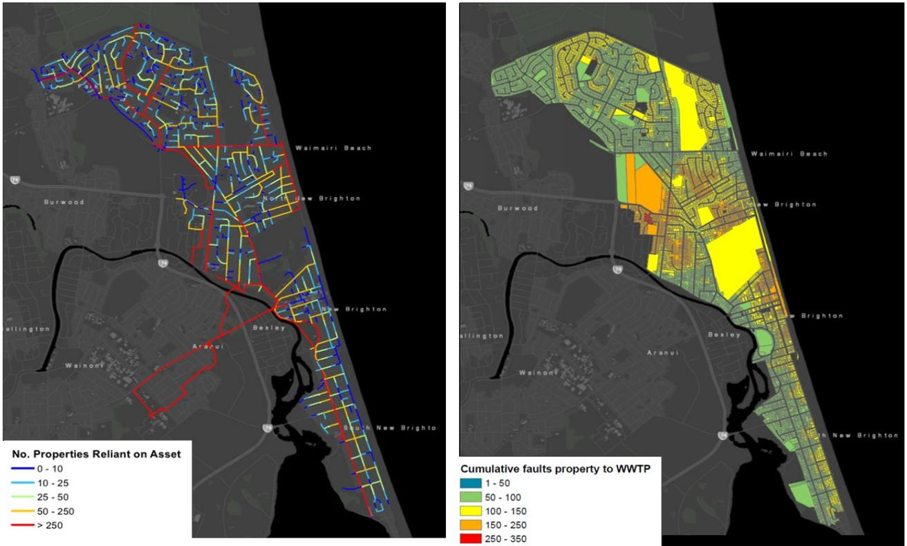
Figure 5: Example of output from assessment of asset criticality, pipe fault index as applied to an eastern area of Christchurch (Beca study completed for Christchurch City Council)
