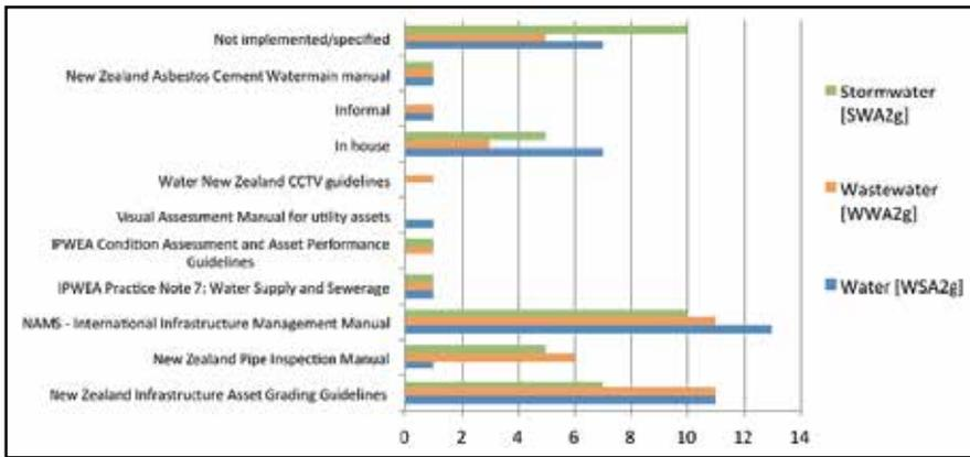
Figure 1: Approaches used for pipeline condition assessments.
