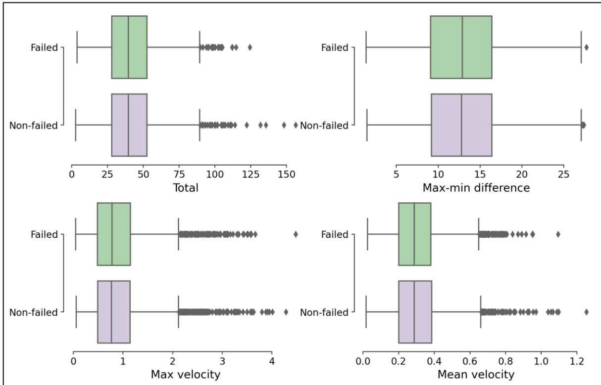
Figure 10: Comparison between failed and intact pipes for all four evaluation criteria
