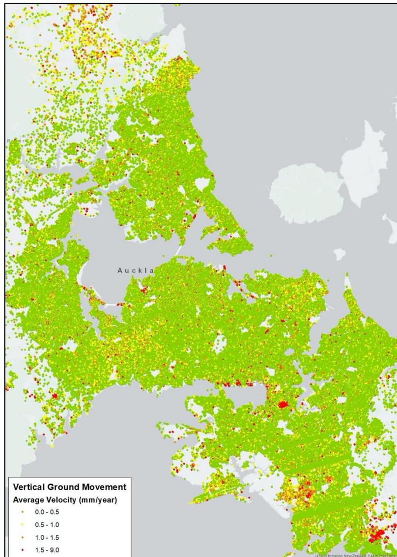
Figure 4: Average vertical ground movement velocity of scatter points in the ground movement dataset.
