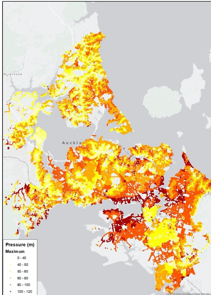
*Figure 3: Distribution of maximum modelled pressure in Auckland's water distribution network*
