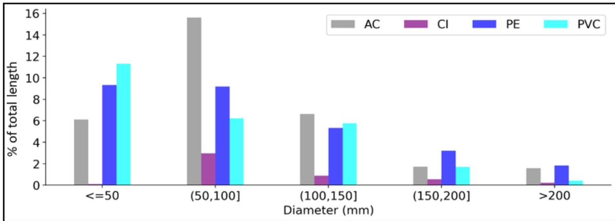
Figure 2: Material profile in Auckland's water supply network.
