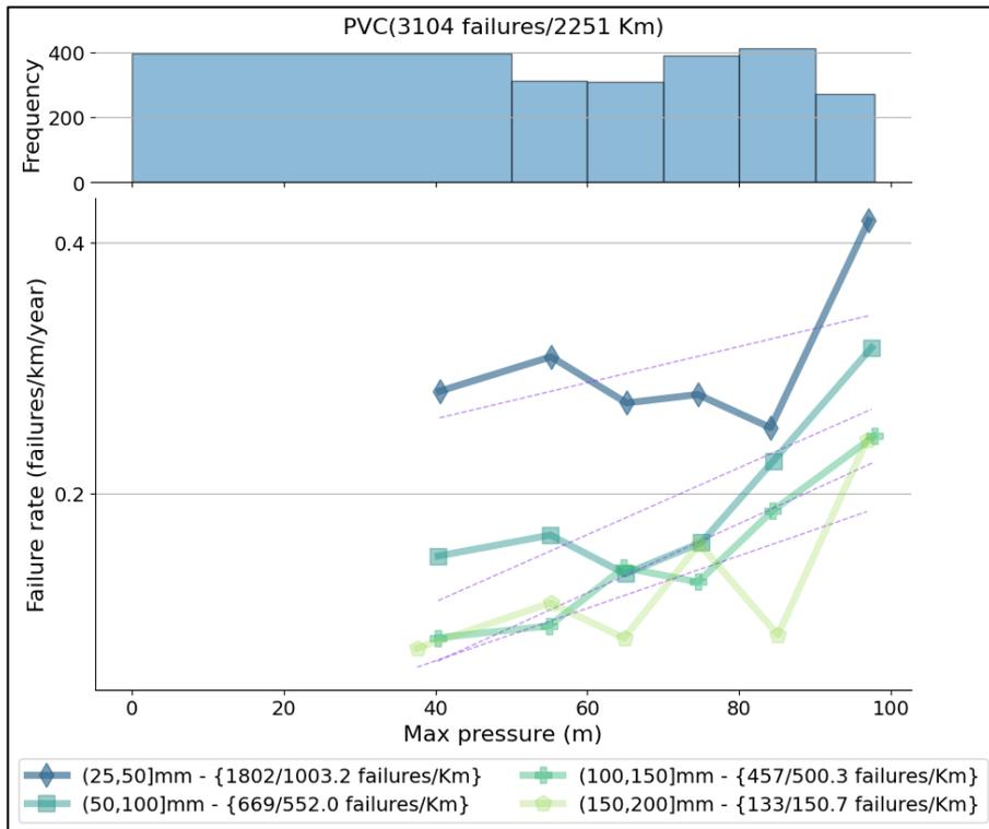
Figure 8: Failure rate against maximum pressure in PVC pipes
