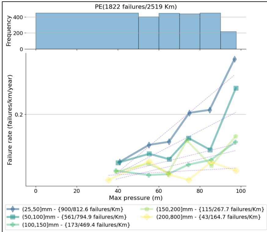
Figure 7: Failure rate against maximum pressure in PE pipes
