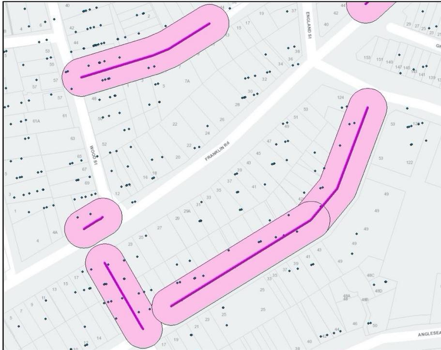
*Figure 9: Intersect between the failed pipes dataset and points of the ground movement dataset.*
