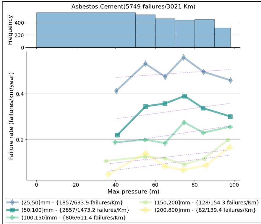
Figure 6: Failure rate against maximum pressure in AC pipes.
