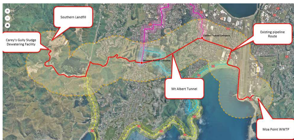
Figure 1: Overview of key Wellington sludge management infrastructure, including Moa Point WWTP, Carey's Gully SDP and sludge transfer pipeline
