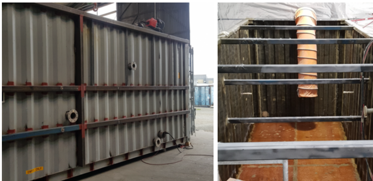
Figure 6 Structural Reinforcing and Fibre Glassing of Containers
