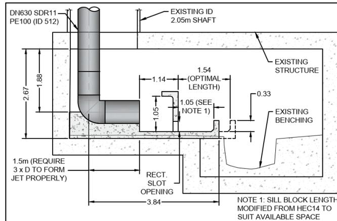
2. A HEC- stilling well was also considered (refer Figure 10). This type of energy dissipator was attractive in terms of its simplicity. The diameter was feasible, but the required height meant there was insufficient clearance between the top of the well and the chamber roof, so this option was also discounted.
