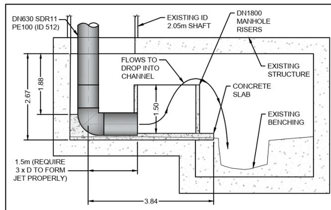
3. A counter-current arrangement (preferred) as described in 3.2.3 below, promised a lower structure height and easier maintenance access.
