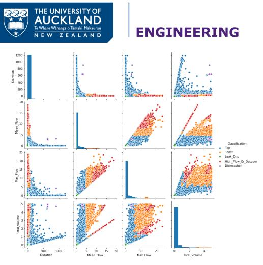
Figure 15 Training data for SVM model, for all events with a total water use volume smaller than 5 litres.
