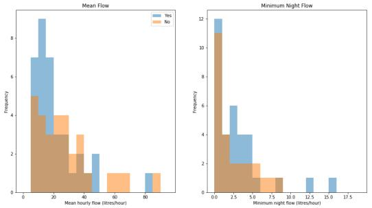
Figure 17 Mean and minimum night flow distributions across all dwellings, considering whether the dwelling was metered and volumetrically charged ("Yes", blue colour) or was not ("No", orange colour).
