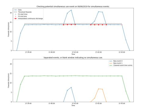
Figure 12 Separation of simultaneous use events: Removal of two short events from a longer event with a consistent discharge.
