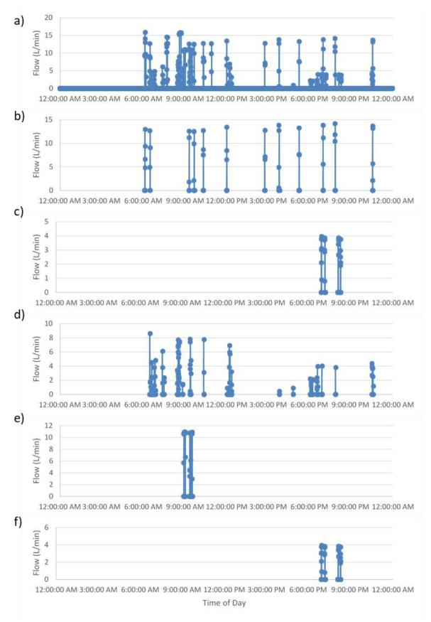
Figure 8 Results of the time series water use disaggregation for one representative Winter day within the overall 2-week period. a) Total water use, including all events; b) Toilet events; c) Shower events; d) Tap events; e) Washing machine events; f) Dishwasher events.
