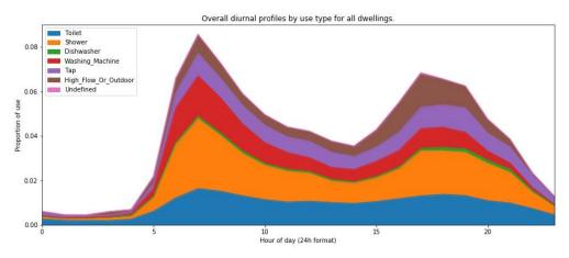
Figure 26 Hourly fluctuations in water use, broken down by use type and averaged across all dwellings.
