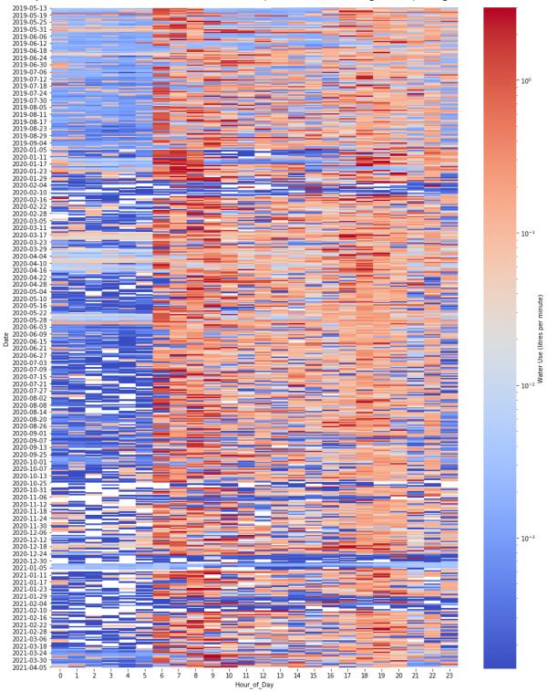
Figure 37 Heatmap plot to enable the identification of leaks within the water use dataset, using a logarithmic colour scale to facilitate easier identification of small leaks or drips. All zero or missing values are denoted by a white colour.
