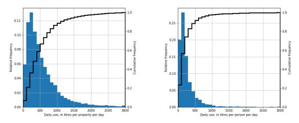
Figure 3 Distributions of daily water use volumes on a per-dwelling (left figure) and per-person (right figure) basis.
