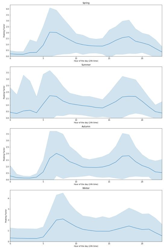
Figure 30 Seasonal variation in peaking factor diurnal curves, where the shaded area represents one standard deviation.
