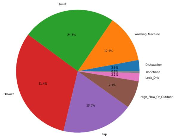
Figure 22 End uses identified from event-based analysis.
