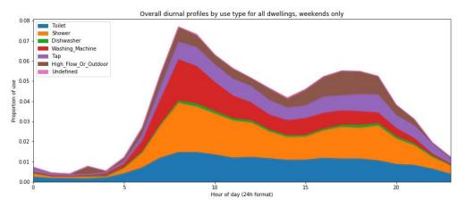
Figure 28 Hourly fluctuations in water use during weekends, broken down by use type and averaged across all dwellings.
