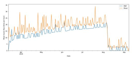
Figure 19 Mean flow and MNF over a long period in time, providing evidence of a possible progressive leak.
