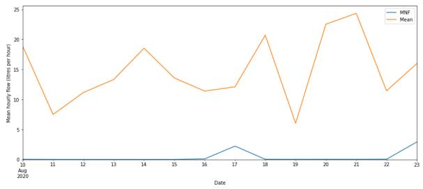
*Figure 10 Daily mean and minimum night flows for a fortnight in Winter for Dwelling 25. During this period, the mean flow was 14.8 litres per hour, while the minimum night flow was 0.4 litres per hour.*
