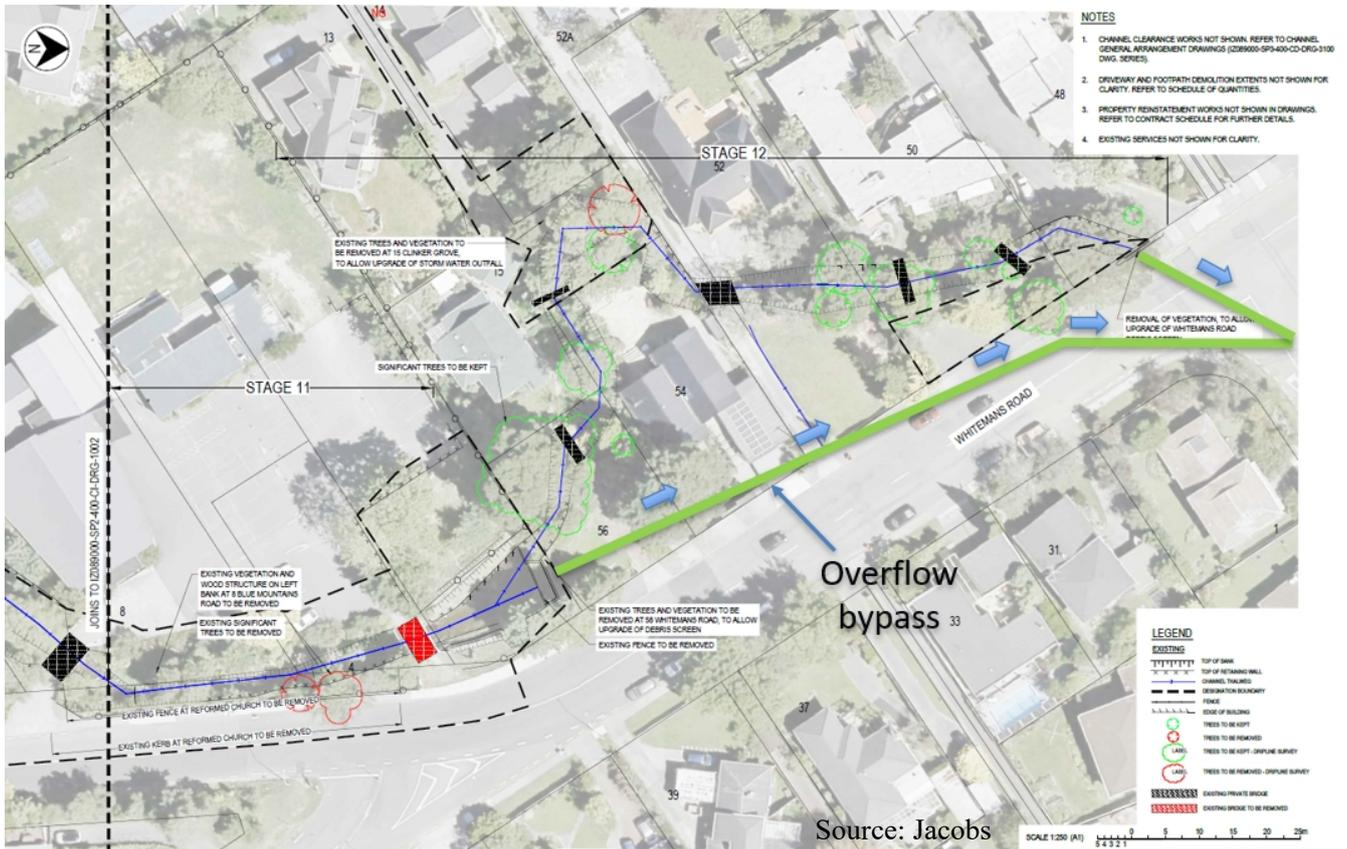
The removal of Stage 11 and 12 from the project provided significant cost savings for the project and a more sustainable solution due to the significant reduction in earthworks and materials for stream retaining structures.
